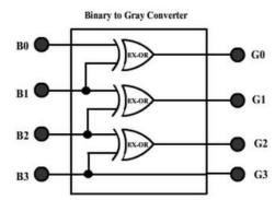
• So that's a simple three EX-OR gate circuit that converts a 4-bit input binary number into its equivalent 4-bit gray code. It can be extended to convert more than 4-bit binary numbers.
