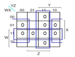
F(W,X,Y,Z)=(W'+X')(Y'+Z')(X'+Z)Or, F(W,X,Y,Z)=X'Y'+X'Z'+W'Y'ZWhich one is the minimal one?
