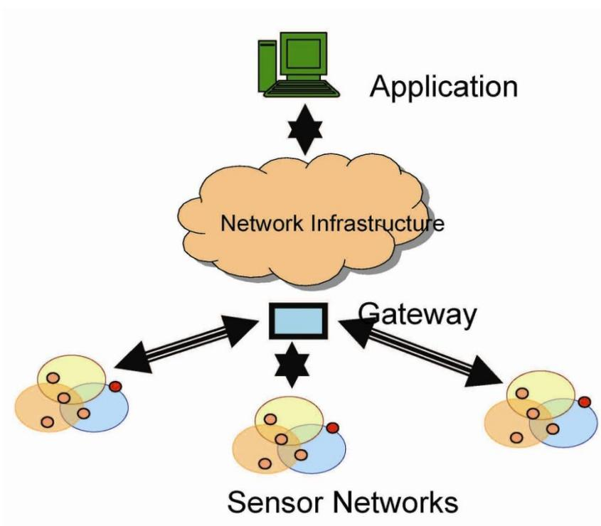
Figure:1.1 Overview of wireless sensor network
