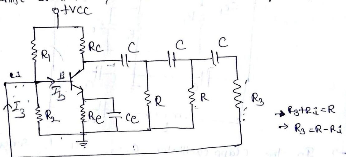
The approximate hybrid-equivalent circuit is given by.
