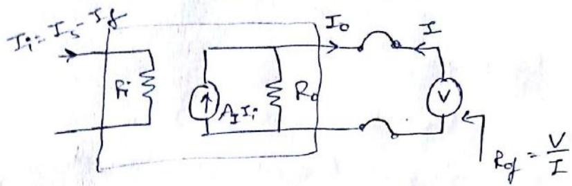
from KCL at output node,  $I + A_I I_i - \frac{V}{R_o} = 0$
