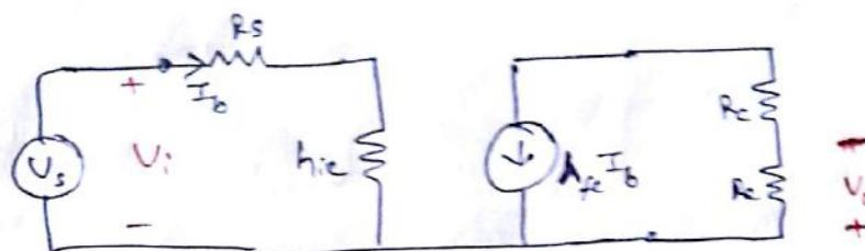
$$A_v = \frac{V_o}{V_i} = \frac{h_{fe} I_b R_c}{V_s} = \frac{h_{fe} I_b R_c}{I_b (R_s + h_{ie})} = \frac{h_{fe} R_c}{R_s + h_{ie}}$$
