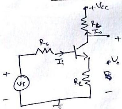
S<sub>1</sub>: The feedback signal is the voltage,  $V_f$ , across  $R_E$ , which is in series with the applied input signal,  $V_S$ .
