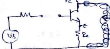
Now  $R_E$  appears in o/p side only, as there is no ip Current ( $I_B = I_E = 0$ ) is flowing
