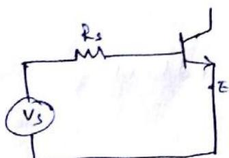
(b) To find the output ckt, set  $I_B = 0$  for Series Mixing.
