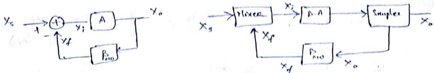
The function of mixer is to <sup>Add/subtract</sup> ~~Combine~~ feedback signal with applied input signal ( $x_s$ ).
