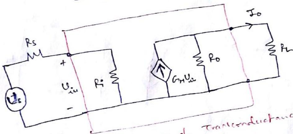
Fig: Equivalent circuit of Transconductance Amp
