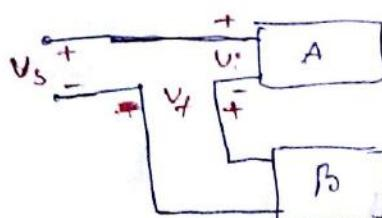
(b) If the feedback signal is in parallel with the external i/p signal, then it is shunt mixing.
