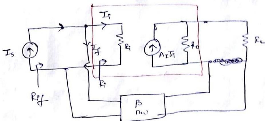
(a)  $R_{if} = \text{input impedance with FB} = \frac{V_i}{I_s}$
