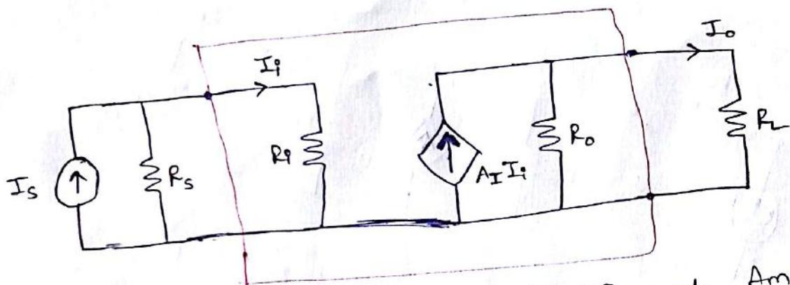
Figs: Equivalent circuit of Current Amplifier.
