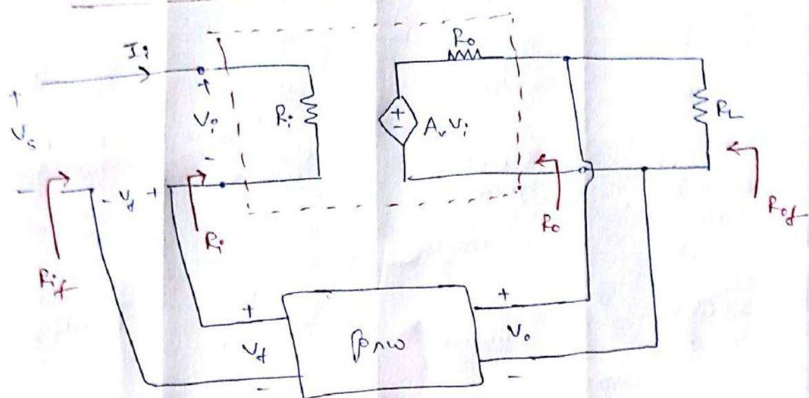
(a) Since the feedback signal  $V_f$  opposes  $V_s$ , the input current
