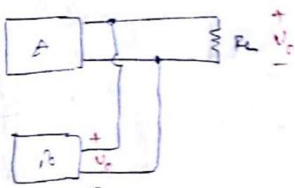
(b) If the sampled signal is taken from the o/p loop, then it is a current sample i.e. if one terminal of the output active device is driving the load and the other terminal is attached to the feedback network then the output sampler is series.
