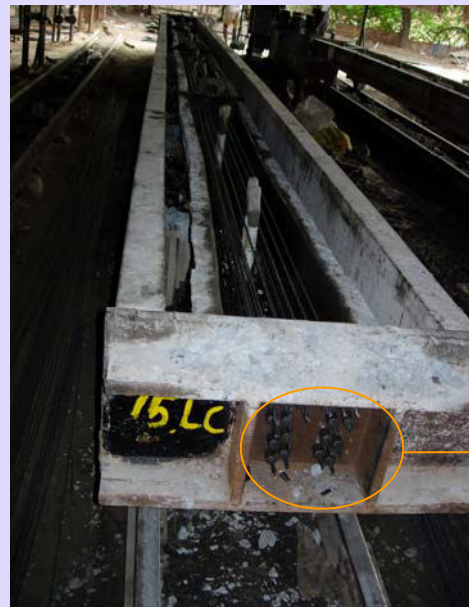
(b) Anchoring of strands
