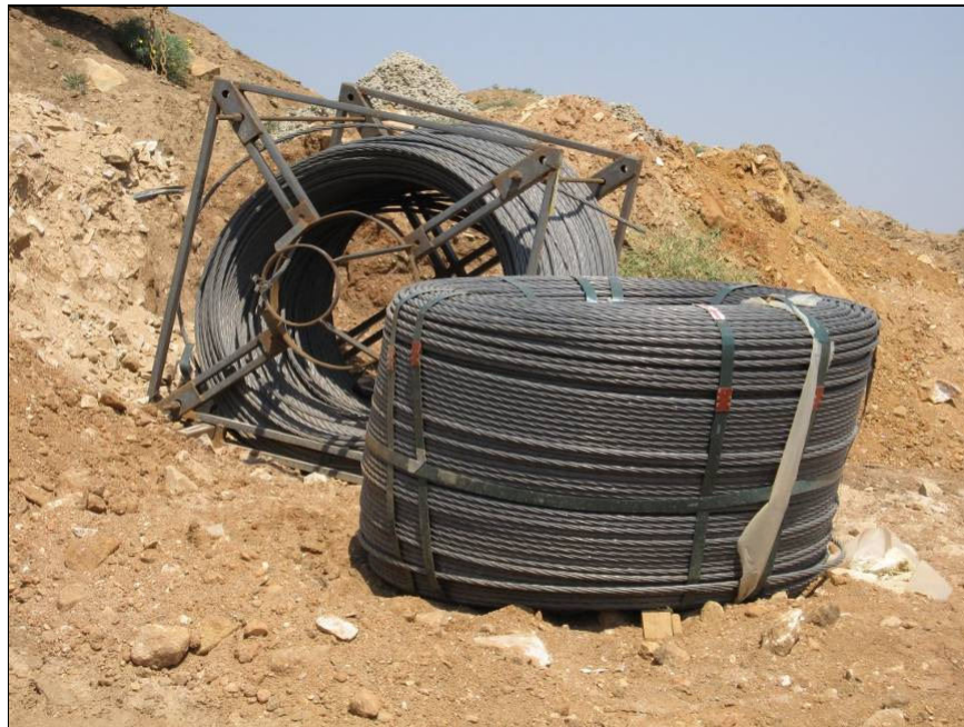
Photo 9.2: Storing of cheeses of prestressing strand: Prestressing should not be stored as shown in the photograph
