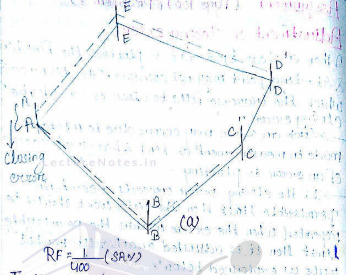
In this case the traverse fails to close by a distance  $A'$ , which is the closing error. To adjust, this error a horizontal  $AA'$  is drawn to represent the perimeter of the traverse to another scale ( $\frac{1}{2000}$ ). On this line distances  $AB_1$ ,  $B_1C_1$ ,  $C_1D_1$ ,  $D_1E_1$  are set off according to the corresponding measured length of the traverse legs.
