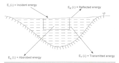
Basic interactions between Electromagnetic Energy and a water body.
