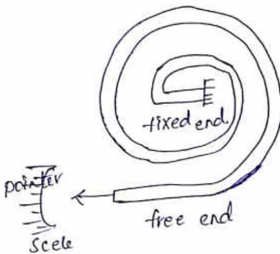
For visual indication, at the free end of strip - a pointer with scale is mounted which gives direct indication of temp on calibrated scale. To get electrical output, LVDT can be used.
