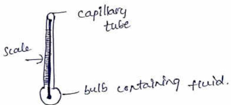
When the temp of the surrounding increases, the fluid in the bulb expands along the capillary tube.
