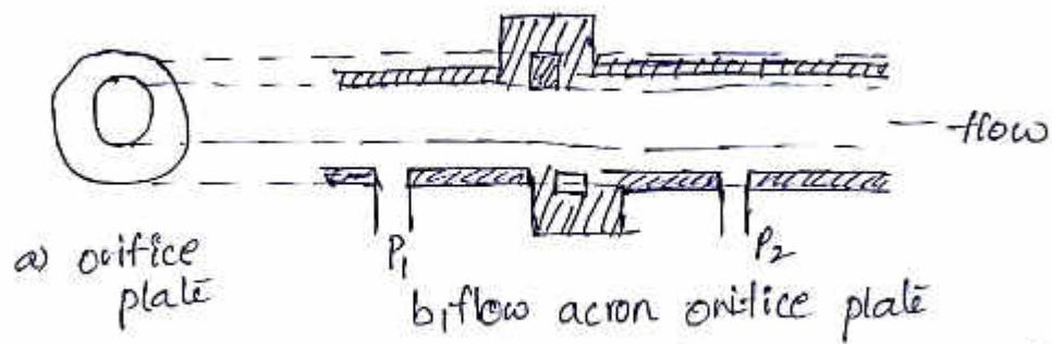
There are certain limitation of the orifice plate. for very high flow rates, the remanent pressure losses are very high. over a period of time, the sharp edges of the hole wear out and the particles in the flowing fluid build up behind the hole reducing the diameter.
