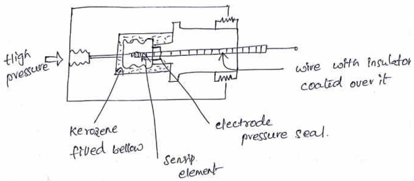
The gold-chrome wire is preferred over manganese wire because its temp sensitivity is lower as compared with that of manganese wire. Over a range of  $40^{\circ}\text{F}$  to  $100^{\circ}\text{F}$ , there is only 0.01% of temp sensitivity for gold-chrome wire.
