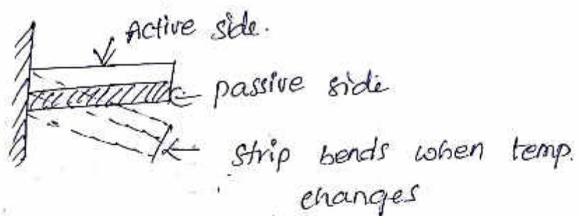
Two metals with different coefficients of expansion are bonded together forming a bimetallic strip unit.
