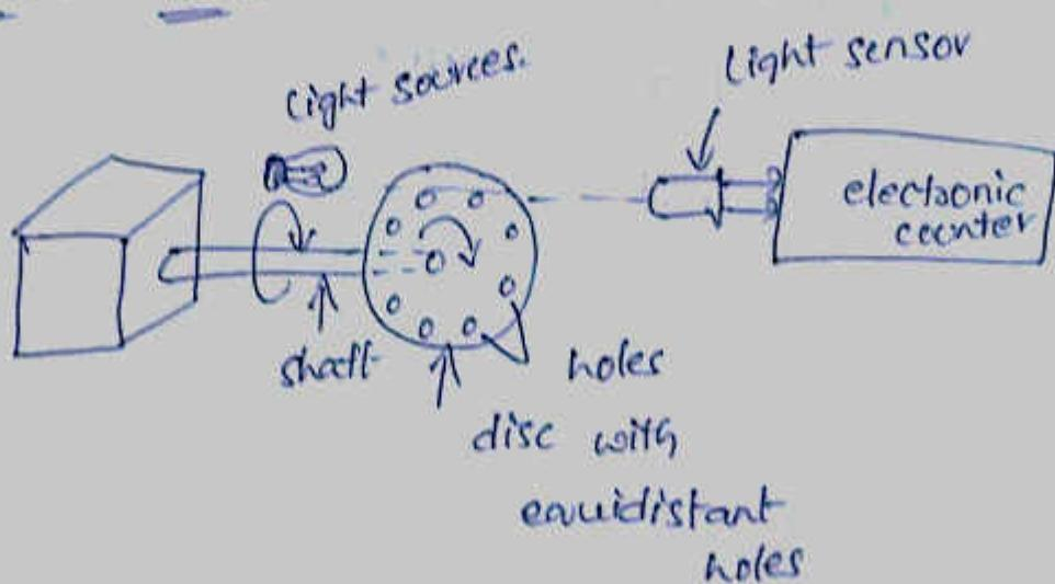
In this method, an opaque disc is mounted on a rotating shaft. Along the periphery of the disc, there are equidistant holes. At one side of the disc, a light source is used. Along the same axis, on other light source.
