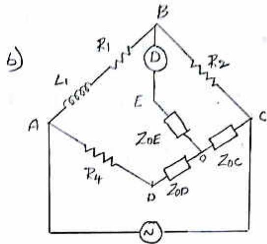
The balance condition for this bridge can be easily obtained by converting the mesh impedances  $R_3, R_5$  to an equivalent star point  $O$  as shown in fig (b).
