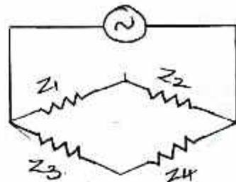
When the bridge is balanced:  $\frac{Z_1}{Z_3} = \frac{Z_2}{Z_4}$
