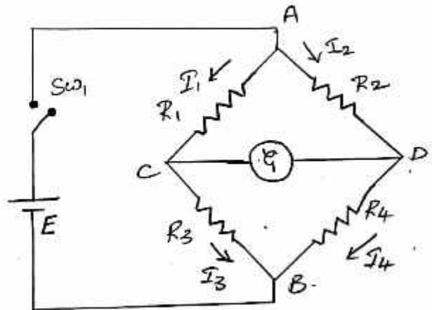
Current in one direction causes the pointer to deflect to one side and in opposite direction to other side.
