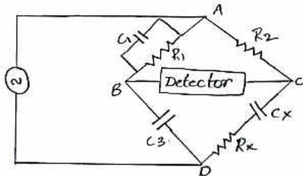
$C_3$  is high quality mica capacitor (low loss) for general measure (or) air capacitor for insulation measurements.
