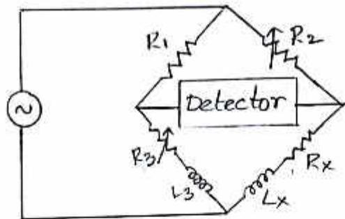
In this unknown inductance ' $L_x$ ' and its internal resistance  $R_x$  are obtained by comparison with standard inductor and resistor  $L_3$  and  $R_3$ .
