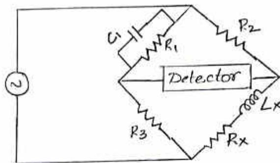
Maxwell's bridge measures an unknown inductance in terms of a known capacitor the use of standard arm offers the advantage of compactness and easy shielding.
