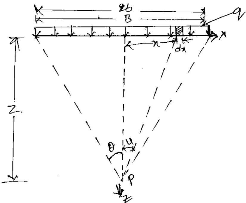
Take an element of width  $dx$  from the distance  $x$  from the centre point of the strip load. The small load of  $q dx$  can be considered as a line load of intensity  $q'$ .
