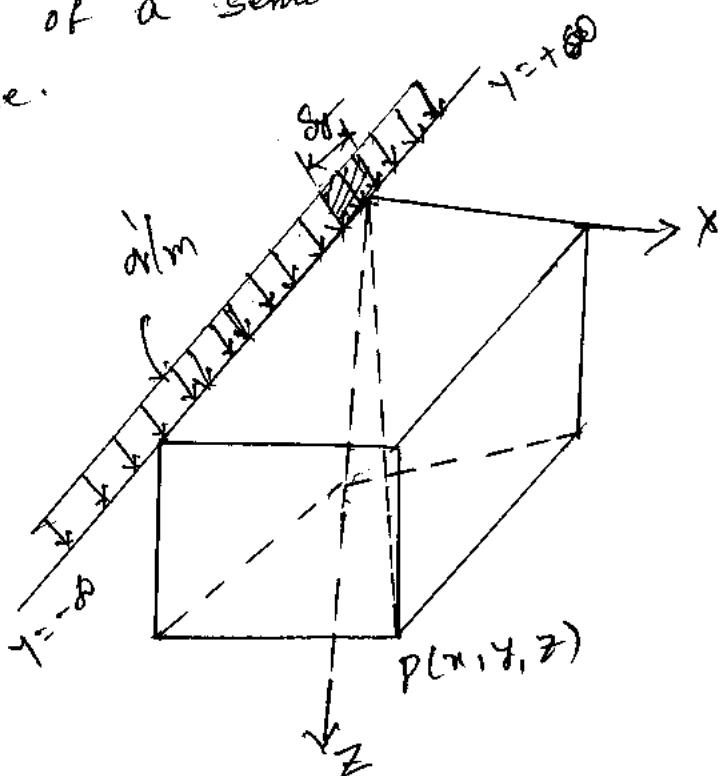
Let us consider the load acting on a small length  $dy$ . The load can be taken as a point load of  $q' dy$  and Boussinesq's solution can be applied to determine the vertical stress at point  $p(x, y, z)$  so the normal stress due to this point load
