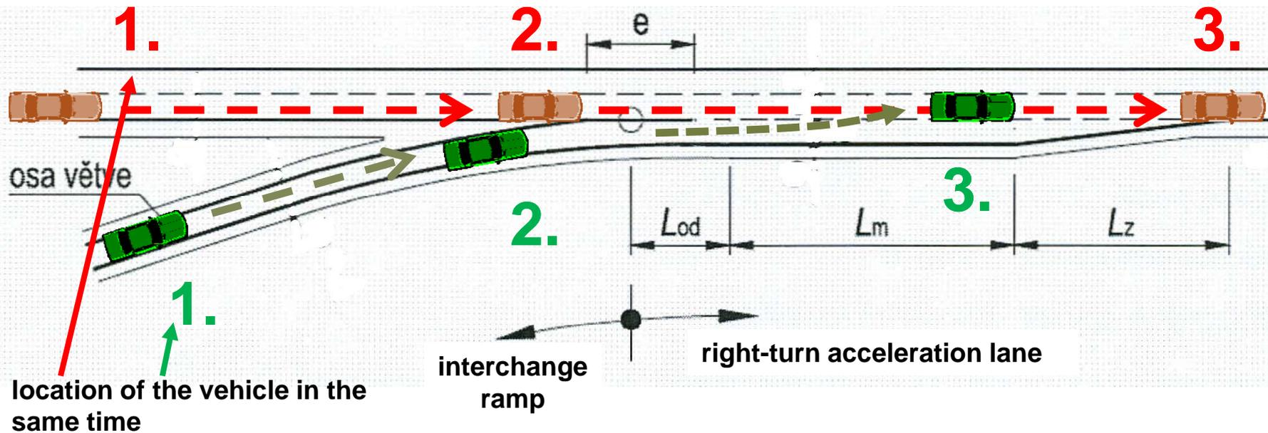
(improvement of traffic continuousness – accelerating vehicles are removed from fast through traffic stream)
