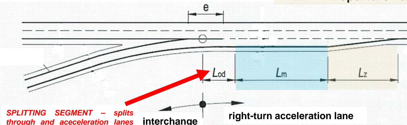
**SPLITTING SEGMENT** – splits through and acceleration lanes (separation line can not exceed to manoeuvring segment)
