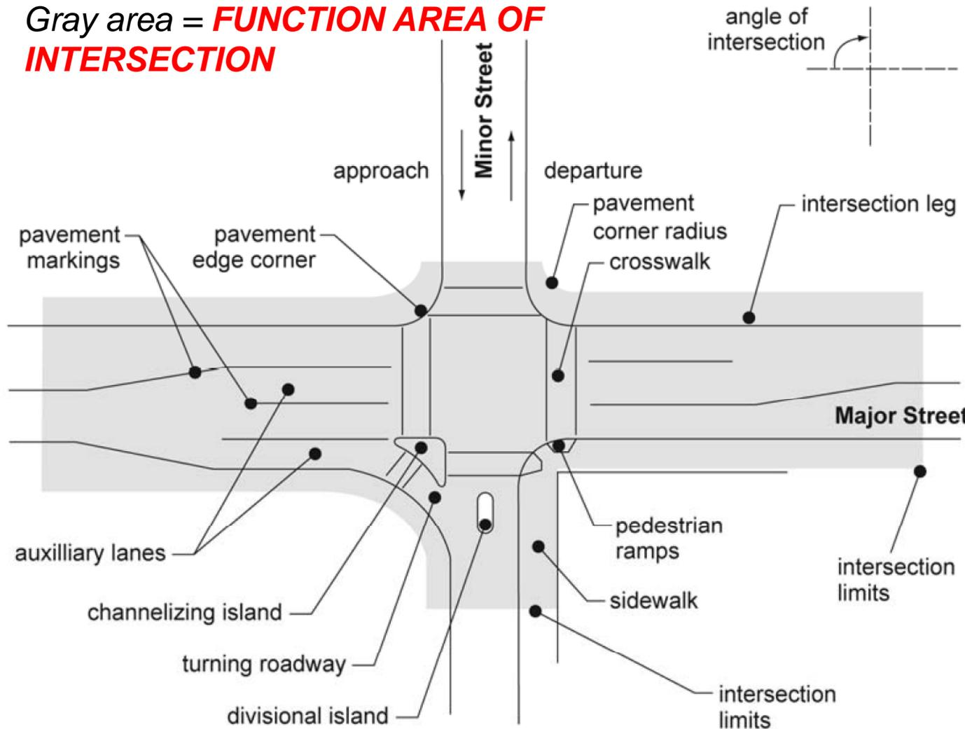
**Sidewalks, crosswalks and pedestrian curb cut ramps** are considered to be within the intersection.
