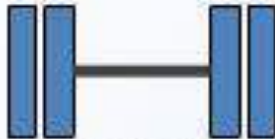
Single Axle With Dual Wheel (Legal Axle Load = 10t)
