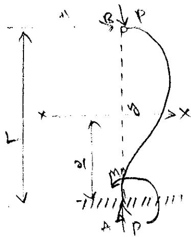
$H$  = Horizontal reaction at B due to  $m_0$  at A
