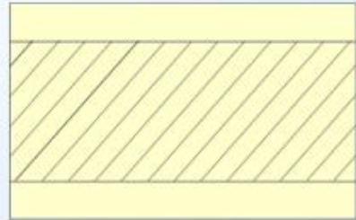
Plaster on Stone Masonry
